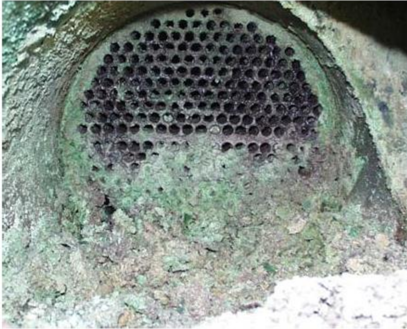
Fig. 13: Sulphuric deposits by undercutting the acid dew point [13]
